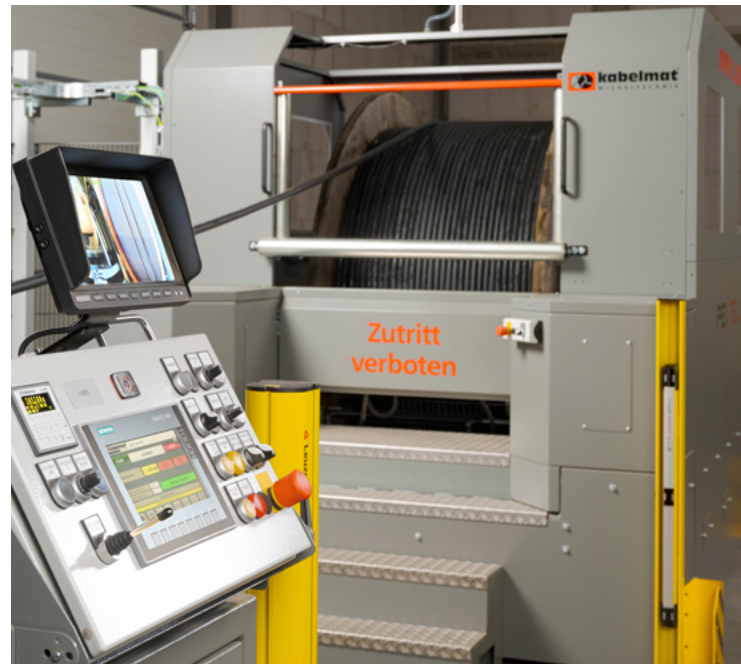
The operator is able to adjust the tensile strength and speed between the two winders using a state-of-the-art touch panel.
