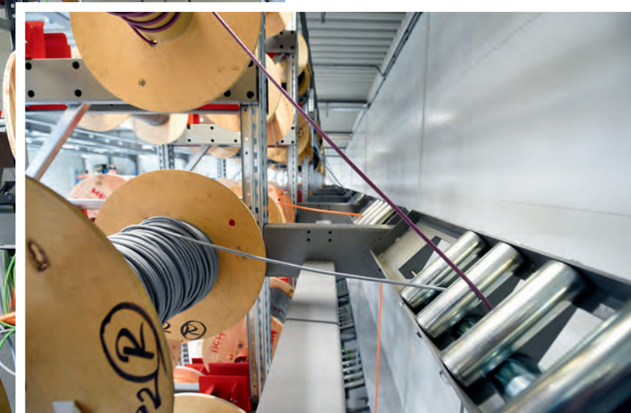
The operator lowers each cable using a pulley, which prevents unused cables from getting in the way when cuts are made.
